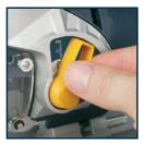
increases the efficiency of cutting. Set the pendulum lever (10) to one of the three settings (1,2 or 3) according to degree of pendulum action required. Experiment on a piece of scrap material to determine the optimum pendulum action setting for the material of the work piece.
